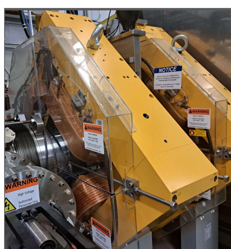
Figure 5: Right: As the largest quadrupole magnet in the beamline, it requires the longest cycling procedure to ensure magnetic field reproducibility. Left: Graph show two procedures for cycling, one that provides reproducible fields within .004% at the cost of a long cycling time, and one faster procedure that reproduces fields within 0.018%. Finding a procedure that minimizes the time and provides reliability is underway.
